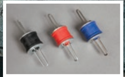
M50R Ceiling Isolation hanger Three variants available with load capacities of 29kg, 54kg and 91kg.
